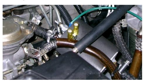
Choose a position along the fuel hose as close to the injector pump as practical. This will hopefully be a point lower than the fuel hose before it, as the glow plug may burn out if air accumulates in the heating unit, especially at start up.
