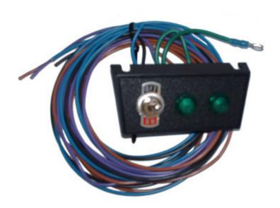
The switch requires an active power source that only comes on when the ignition is in the on position, as we want the heating elements to turn off when the ignition is off. There are many places that you could "pick up" a supply with the most universal being at the cigarette lighter or stereo, although the switch may then also operate in the accessories position.
