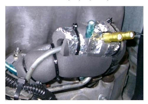
that the thermostat housing is under the tube cover and the edge of your cut is "kissing" the black section of the thermostat.
