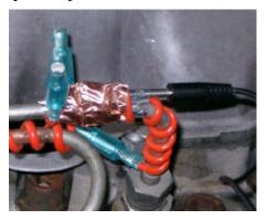
will make direct contact with both loops of the element. The thermometer probe will assist to make a flat spot for mounting. Wrap a piece of copper tape around the element at this point. Remember that the heating element has to transfer the heat to the thermostat via the copper tape so a thin layer is suggested.
